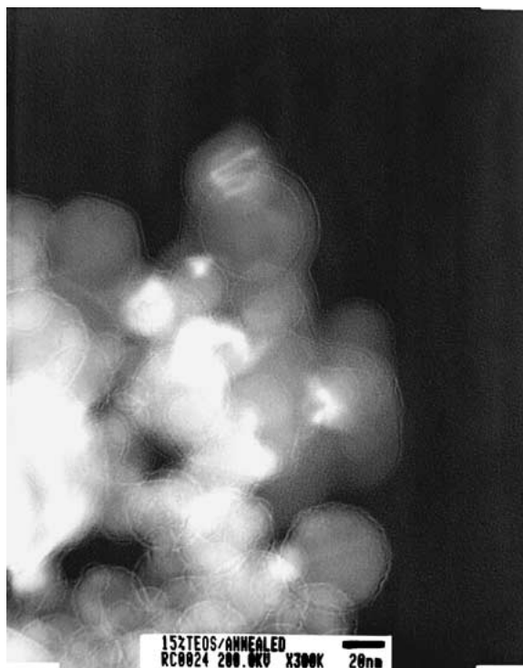
Figure 3 Transmission electron micrograph of the 15% glass-coated \delta -alumina.
